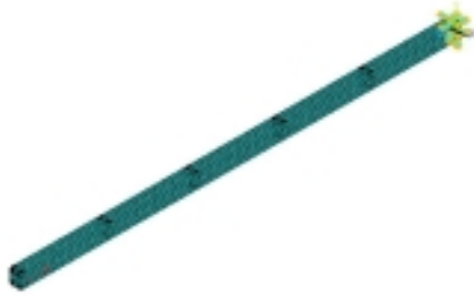
c) Spar eccentrically loaded FEM mesh
