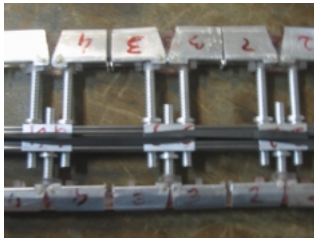
Figure 16: Detail of the rubber strings in the final mechanism assembly
